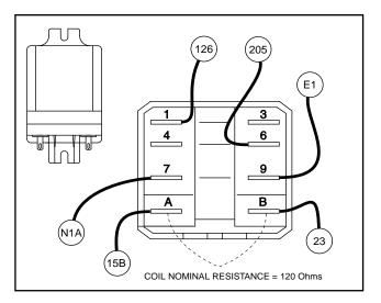
Figure 3. Transfer Relay Test Points
